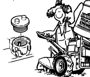
Change oil at regular intervals using a a high quality oil such as Snapper's small engine formulated 4-cycle engine oll. Refer to the engine owner's manual for oil details.
